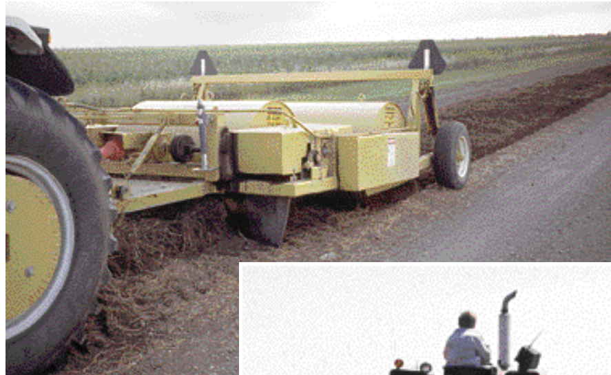
Windrow pulverizer fabricated by the Hyde County Highway Department of Highmore, South Dakota.
